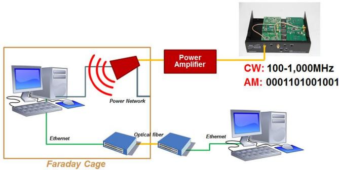
Figure 2: Experimental set-up for the radiated case.
