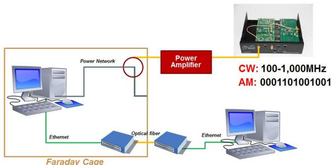
Figure 4: Experimental set-up for the conducted case
